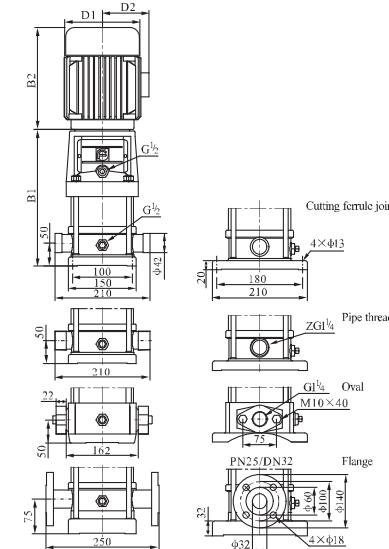
CDL5-18~24 sub-connection of pipeline has no oval flange connection.
