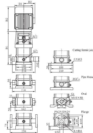
CDL2-13 ~ 18 sub-connection of pipeline has no oval flange connection.
