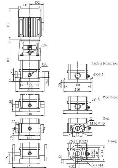
CDL1-19 ~ 25 sub-connection of pipeline has no oval flange connection.
