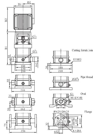
CDL3-17 ~ 3-25 sub-connection of pipeline has no oval flange connection.
