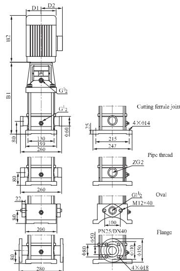
CDL8-10~8-14 sub-connection of pipeline has no oval flange connection.
